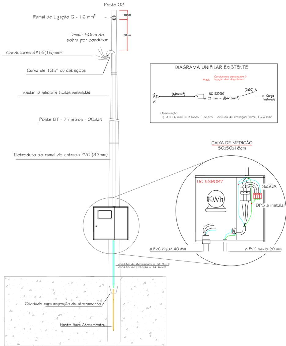
**Diagrama Unifilar A INSTALAR**
